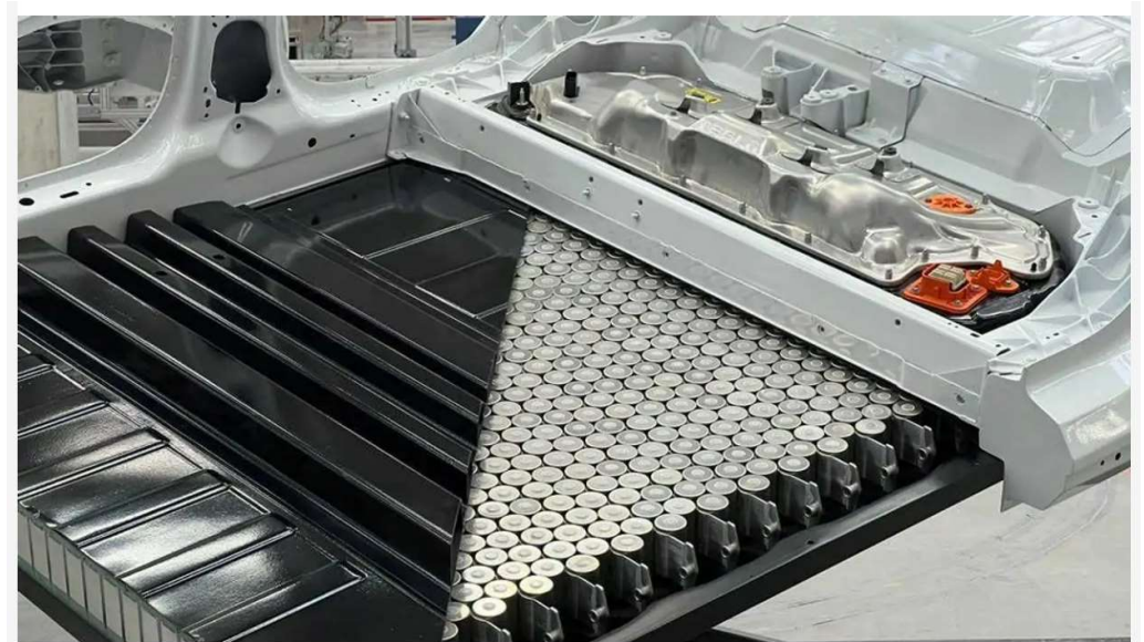
Tesla battery with cylindrical cells (46mm diameter; 60mm height)
