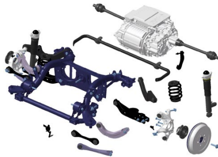
e.g. 5-control-arm axle with electric drive
